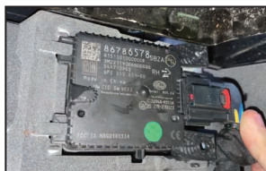
Figure 2: The module is installed facing the correct direction.
