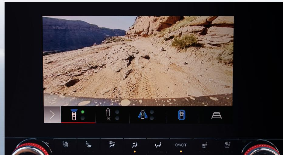
(clear lane markings, clean windshield, vehicle speeds maintained between 35–56 mph). If these conditions are not met, the front-view camera module will continuously run the service-point calibration until it is successfully completed. The calibration will work across ignition cycles and does not require re-initialization at startup.
